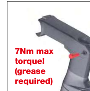
Install stem steerer clamp bolt - grease required!
