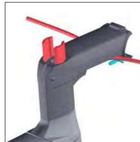
Install stem and steerer inserts
